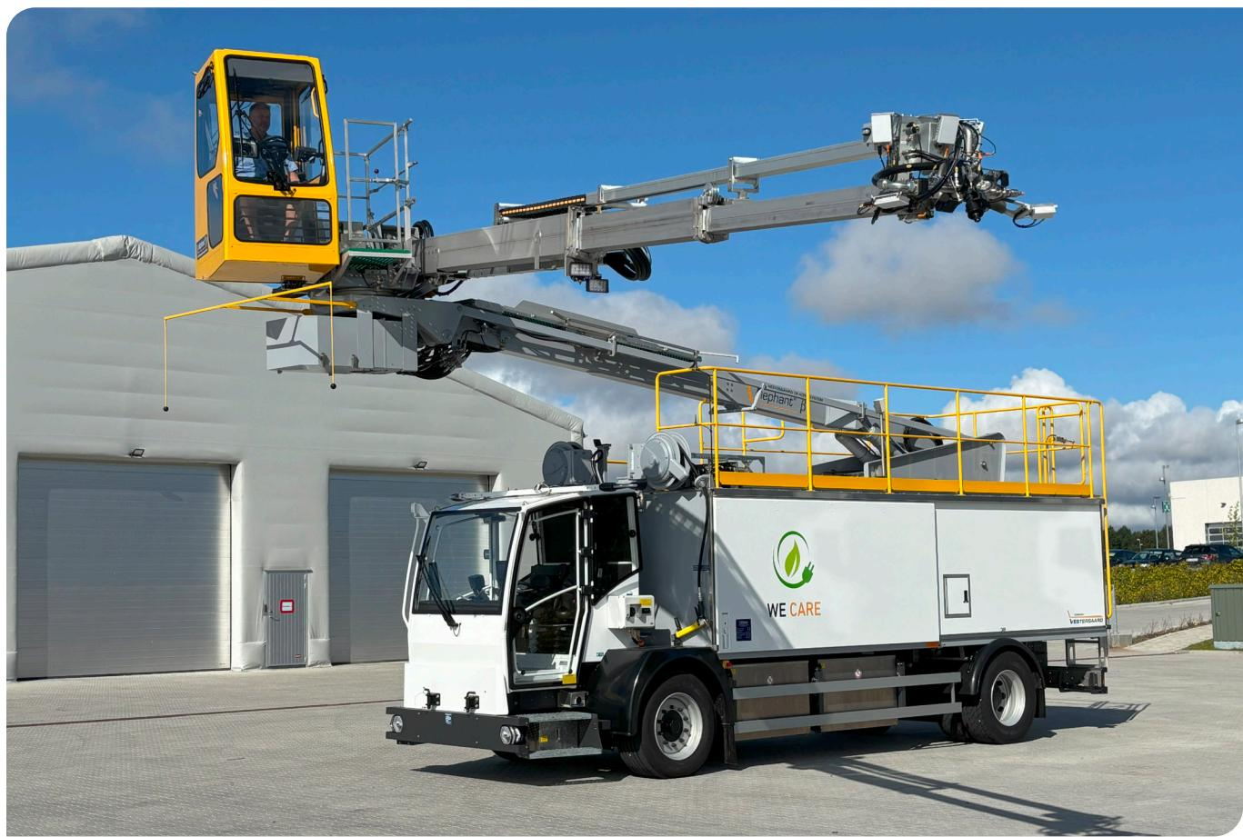
The iconic Elephant® BETA is now available in a Fully Electric version. Built on a Vestergaard electric chassis with 160 kWh battery, the Elephant® e-BETA Fully Electric sports all the well-known efficiency and reliability of the Elephant® BETA.
