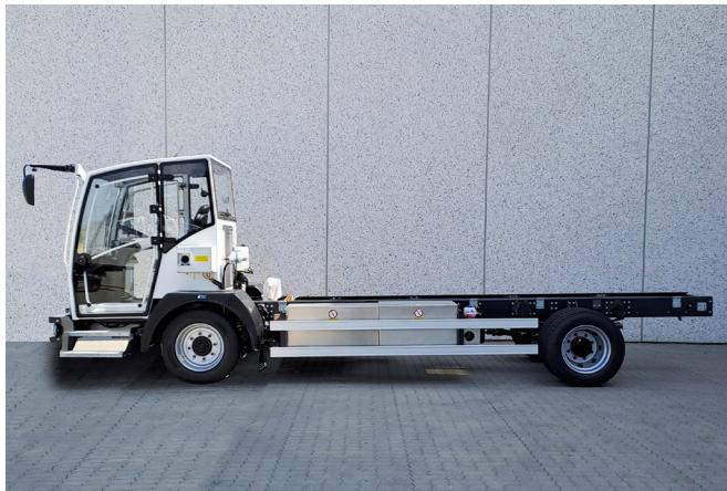
Vestergaard Company's fully electric chassis is able to carry a number of applications, e.g. water and lavatory carts or de-icing units. The smallest version is equipped with a 60 kWh lithium-ion battery with enough capacity to drive up to approximately 50 km and operate for approximately 12 hours. Also available with 70 kWh battery.
