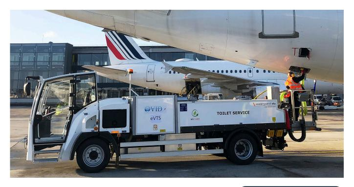
Vestergaard Company has launched the e-VTS - our well-known vacuum toilet service unit - in a sustainable version on a fully electric 9 t chassis. The first version is equipped with a 40 kwh lithium-ion battery with enough capacity to drive up to approximately 50 km and operate for approximately 12 hours. Also available with 60 or 70 kwh battery.
