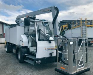
Vestergaard Company has launched the e-Mini MY Lite - our well-known smallest aircraft deicer - in a sustainable version on a fully electric 12 t chassis. The first version is equipped with a 40 kwh lithium-ion battery with enough capacity to drive up to approx. 30 km and up to 15-20 deicing operations on one charge.
