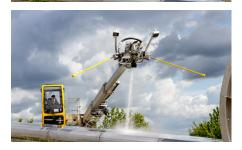
When the operator's cabin is moved up or down the PPS system sensors ensure that the spray distance to the aircraft surface remains the same.
