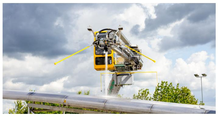
It is a fact of nature that the shorter distance heated fluid has to travel from nozzle to surface the less of a temperature drop. Vestergaard has developed a system which optimizes the distance from the nozzle to the aircraft surface, the patented Precise Positioning System – PPS.
