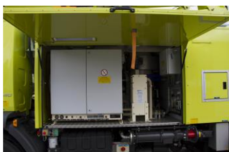
Top-hinged doors on either side of the body provide an easy access to the machine room for service.
