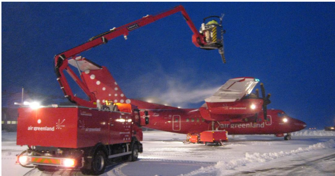
The Elephant ® My provides the customer with the Forced Air System, which ensures highly efficient snow removal with the maneuverable nozzle and the shortest possible blow distance.
