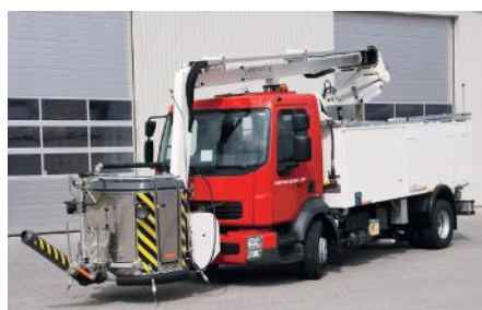
The Forced Air System provides highly efficient snow removal with the maneuverable nozzle and the shortest possible blow distance.
