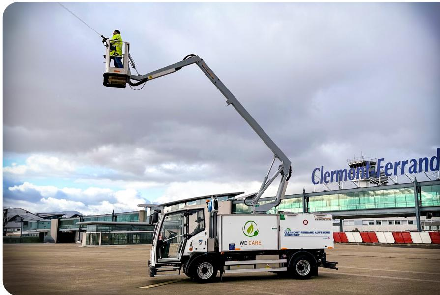
The e-Mini MY Lite is a fully electric deicer on a 12 T chassis. It is equipped with a 60 kWh lithium-ion battery and the heating of the fluid can be accomplished with either an electric system or a conventional diesel heater.
