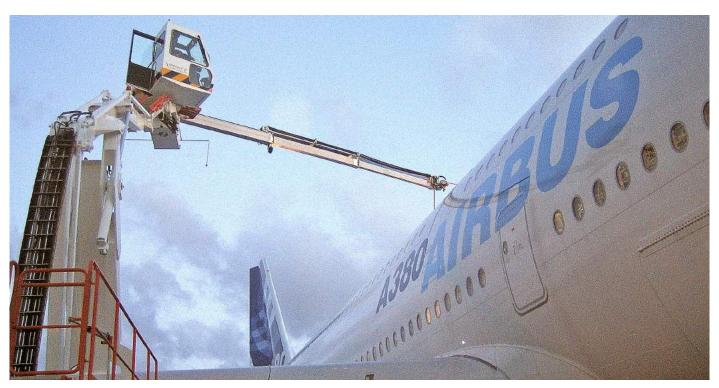
The Elephant® Beta-15 provides customers all over the world with highly efficient, reliable and safe deicing. The extended telescope reduces application time and minimizes movement around the aircraft. The longer telescope also reduces glycol usage.
