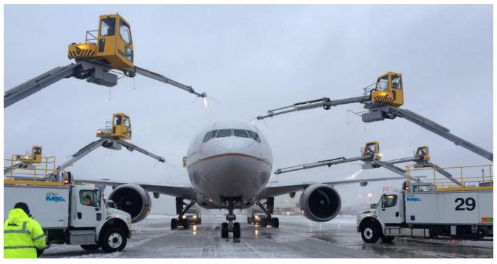
The Elephant® Beta provides customers all over the world with highly efficient, reliable and safe deicing. The extended telescope reduces application time and minimizes movement around the aircraft. The longer telescope also reduces glycol usage.
