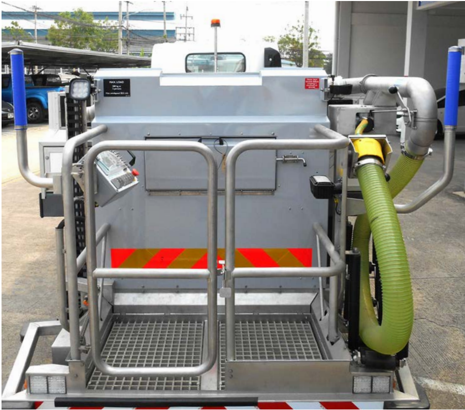
The Vestergaard Water and Vacuum Toilet Service units are equipped with an elevating basket. The spacious basket – with plenty of room for two persons – is easily entered from the ground level.
